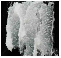
Substance processed with conventional mixing procedure show crystalline substances that are still clearly visible.
